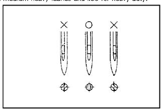
Needle should be set correctly facing their long slot towards operator; mark (X) in fig. 12 shows incorrect setting of needle. While operating machine in high speed, due to the friction occurred between needle and fabric causing stitch skipping, thread broken and the penetrated hole on the fabric will become much bigger, especially when compound thread and fabric are used.
