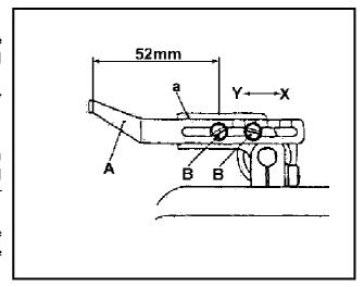
In case of general sewing condition, the distance between the center of screw and thread eyelet of thread guide should be 8mm.
